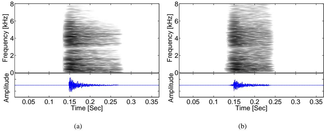
Fig. 1. Transient waveforms and spectrograms. (a) A clean transient (door knock) event. (b) The estimated transient.
