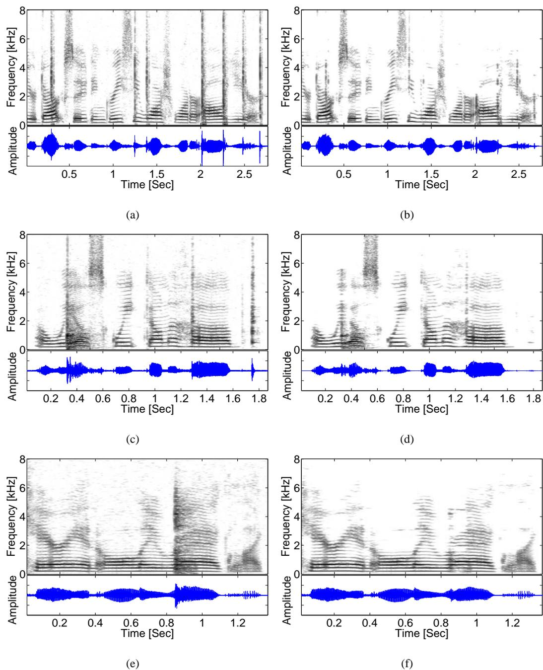
Fig. 2. A segment of the measurements and enhanced signals waveforms and spectrograms. (a) Noisy signal with 7 key strokes. (b) Enhanced speech with suppressed keyboard typing. (c) Noisy signal with 4 events of household interferences. (d) Enhanced speech with suppressed household interferences. (e) Noisy signal with a door knock. (f) Enhanced speech with suppressed door knocks.
