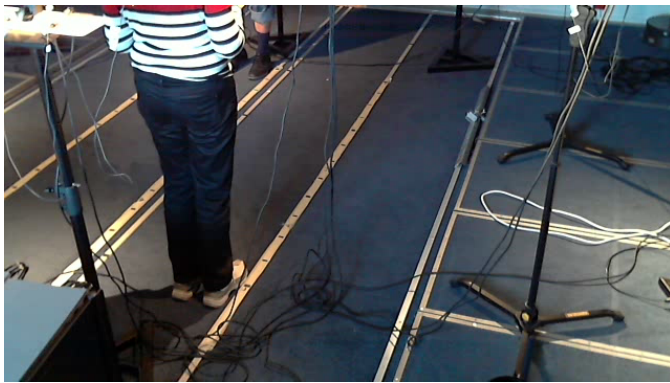
Figure 5. First scenario: low reverberation level( T_{60} = 200 msec); two speakers with a large distance between them.
