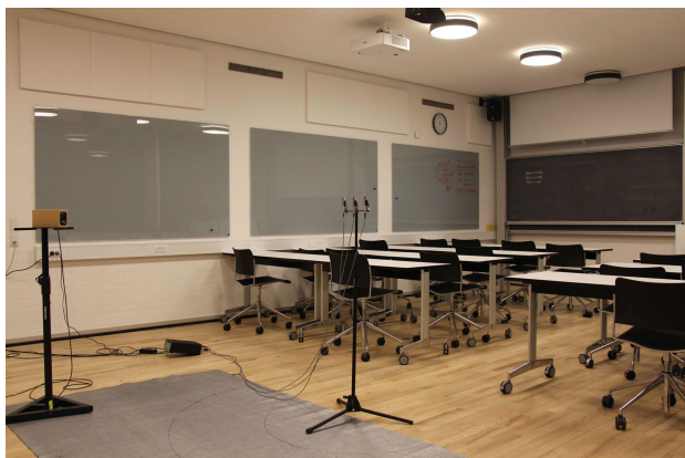
FIGURE 3. Classroom and measurement configuration at Technical University of Denmark (DTU) where room IRs were collected [33].
